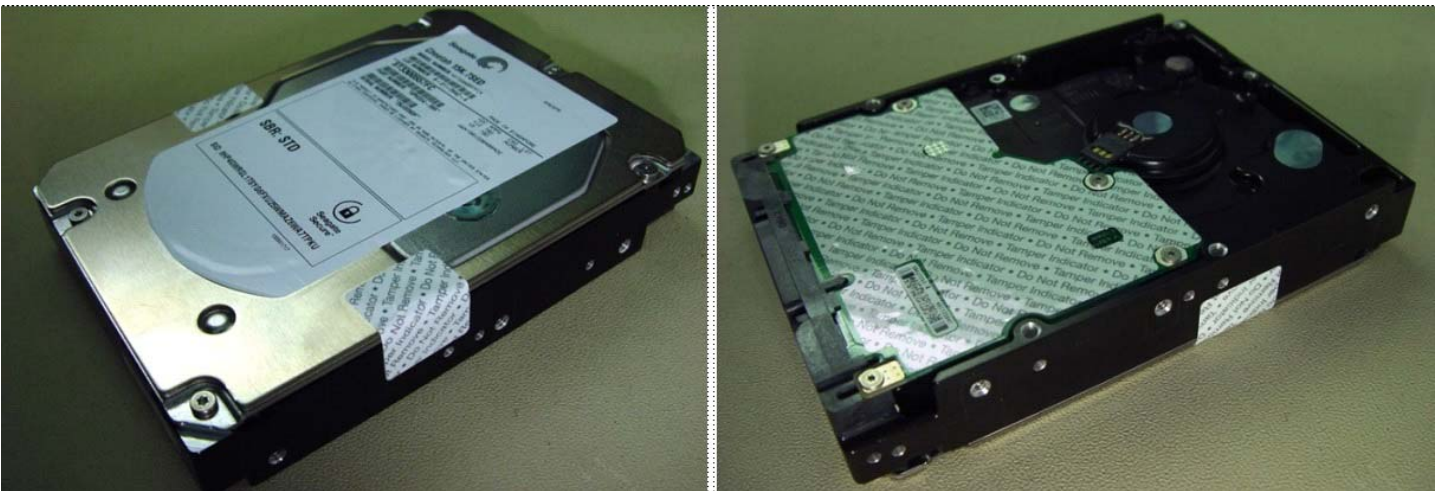
Figure 4. Example of FIPS tamper evidence labels.
