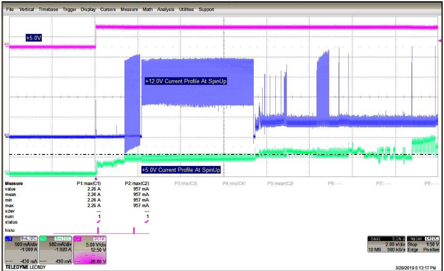
Figure 1. 16TB model current profiles.
