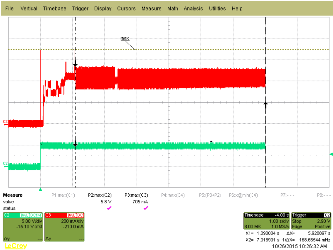
Figure 1. 6TB Typical 5V startup and operation current profile
