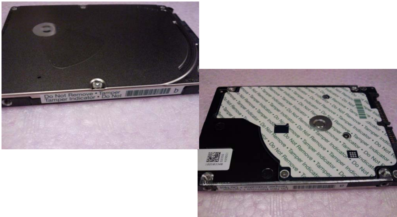
Figure 6. Example of FIPS tamper evidence labels.
